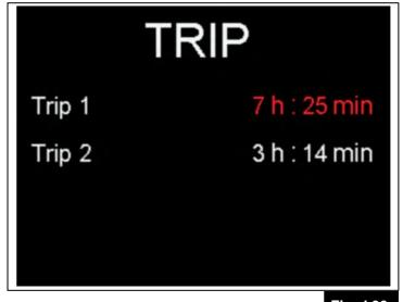
To perform zeroing, press the left button (K1) for 1 second, alternatively press the left button (K1) again to go to the selection of the second item. Following any resetting of the first item, the selection will automatically switch to the second item.
